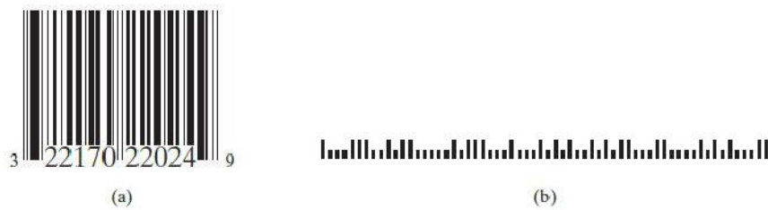
Figure 12.1 Two forms of linear bar codes are (a) width-modulated, exemplified here by the Universal Product Code, and (b) height-modulated, exemplified here by Postnet, used by the U.S. Postal Service.
